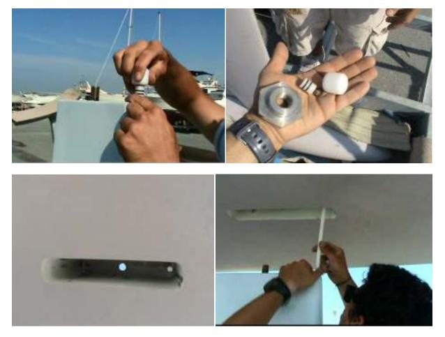
The keel head part is conical. When the boat gets lowered on to keel the keel bolt goes to its hole easily. The weed knife rod should be pulled out and should be stuck into its hole before lowering the boat on the keel.
