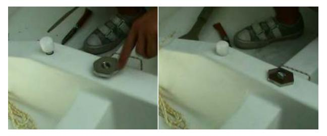
Weed knife can be operated inside of the boat by puling the ball up and pushing it in to its slot
